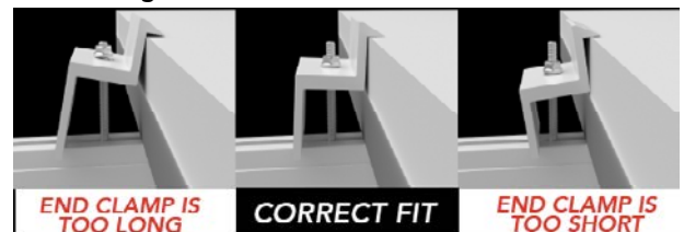
Figure 20. Check End Clamp Fit
