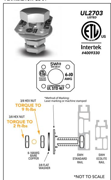
Figure 2. Slide SW-GB-01 grounding bolt into side mounting slot of rail. Tighten inner hex nut to 9 ft-lbs. Nibs will penetrate rail anodization and create grounding path through rail. Slide bare copper wire into cutout slot of grounding bolt. Tighten outer hex nut to 2 ft-lbs to bond bare copper wire between the two hex nuts.
