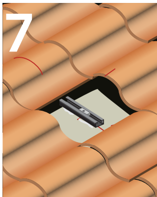
STEP 7: Slide channel nut to line up with the crown of tile.
