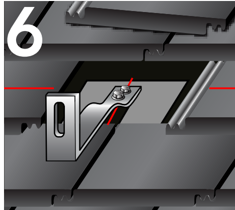
STEP 6: Insert lag bolts through 5/16" SS flat washers and into rafter.
