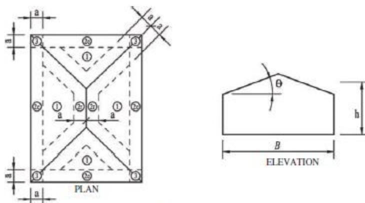
FIGURE 30.3-2H Components and Cladding [ $h \leq 60$  ft ( $h \leq 18.3$  m)]: External Pressure Coefficients, ( $GC_p$ ), for Enclosed and Partially Enclosed Buildings—Hip Roofs,  $27^\circ < \theta \leq 45^\circ$  (Roof)
