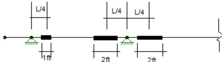
Continuous Span (3 spans or greater)
