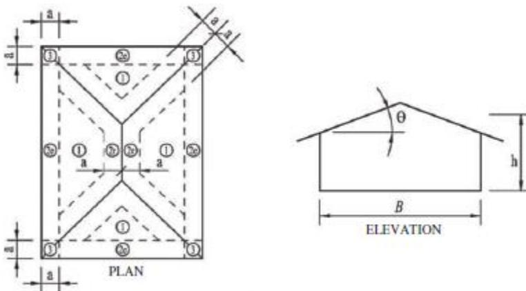
FIGURE 30.3-2G Components and Cladding [ $h \leq 60$  ft ( $h \leq 18.3$  m)]: External Pressure Coefficients, ( $GC_p$ ), for Enclosed and Partially Enclosed Buildings—Hip Roofs,  $20^\circ < \theta \leq 27^\circ$  (Roof and Overhang)
