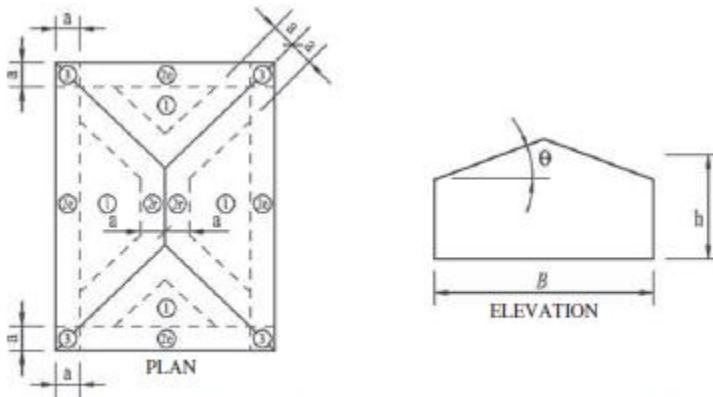
FIGURE 30.3-2E Components and Cladding [ $h \leq 60$  ft ( $h \leq 18.3$  m)]: External Pressure Coefficients, ( $GC_p$ ), for Enclosed and Partially Enclosed Buildings—Hip Roofs,  $7^\circ < \theta \leq 20^\circ$  (Roof)
