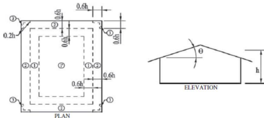
**FIGURE 30.3-2A Components and Cladding [ $h \leq 60$  ft ( $h \leq 18.3$  m)]: External Pressure Coefficients, ( $GC_p$ ), for Enclosed and Partially Enclosed Buildings—Gable Roofs,  $\theta \leq 7^\circ$**
