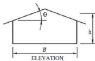
FIGURE 30.3-2B Components and Cladding [ $h \leq 60$  ft ( $h \leq 18.3$  m)]: External Pressure Coefficients, ( $GC_p$ ), for Enclosed and Partially Enclosed Buildings—Gable Roofs,  $7^\circ < \theta \leq 20^\circ$
