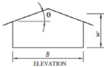
FIGURE 30.3-2C Components and Cladding [ $h \leq 60$  ft ( $h \leq 18.3$  m)]: External Pressure Coefficients, ( $GC_p$ ), for Enclosed and Partially Enclosed Buildings—Gable Roofs,  $20^\circ < \theta \leq 27^\circ$
