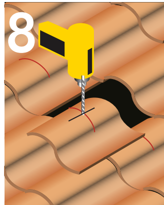
STEP 8: Using 3/8" carbide bit and a rotary hammer, drill through the crown of the tile at the intersection
