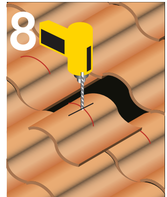
STEP 8: Using 3/8" carbide bit and a rotary hammer, drill through the crown of the tile at the intersection
