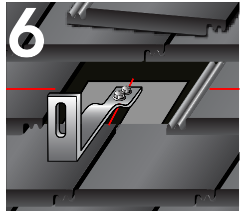
STEP 6: Insert lag bolts through 5/16" SS flat washers and into rafter.
