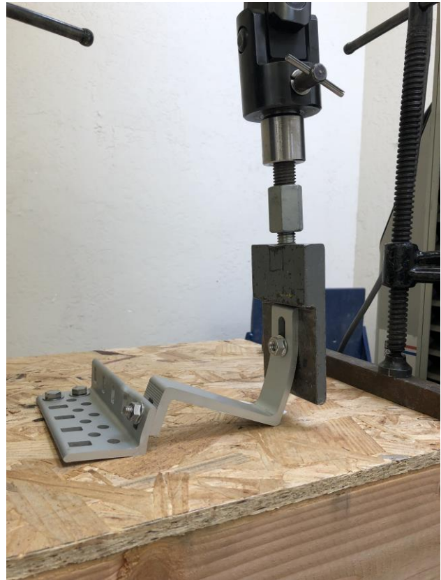
Figure B1b. Typical Failure Mode
