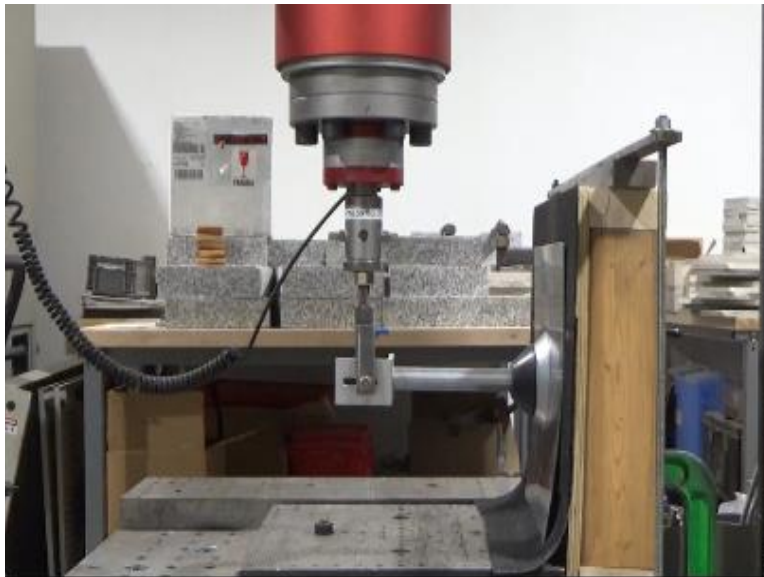
Photo No. 6 ASTM D1761 Lateral Fastener Resistance Test Setup
