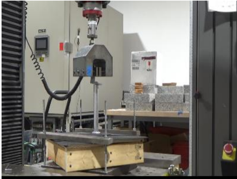
Photo No. 3 ASTM D1761 Fastener Withdrawal at Test End (typical)
