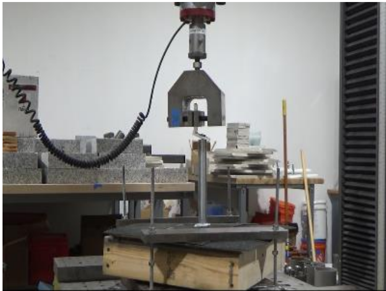
Photo No. 4 ASTM D1761 Fastener Withdrawal at Test End (typical)
