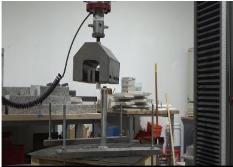
Photo No. 2 ASTM D1761 Fastener Withdrawal Test Setup
